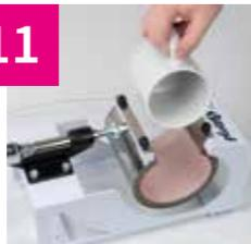
As soon as the countdown ends, a repeating signal tone will occur. Press the TIMING Button to stop the countdown and switch off the signal tone. Now open the press and carefully remove the mug by the handle.
