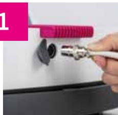
Connect your Mug Press to the iXpress Transfer Press. If the iXpress Transfer Press is connected to an outlet, unplug it before connecting it to the Mug Press.
