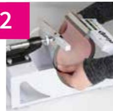
Pull the lever backwards to open the press and remove the attachment from the metal rack.
