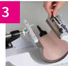
Tip: When inserting a new attachment, make sure that you mount it with both screws on the left side first.
