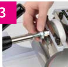
Before using the Mug Press, make sure your mug is firmly placed in the press. Place the mug in the cold press and close it. The mug should now sit firmly in the Mug Press and the press should be completely closed.
