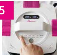
Set the desired temperature (TEMP Button) and time (TIMER Button) on the iXpress Transfer Press.
